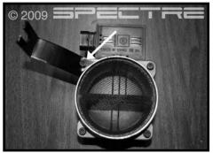
Step 6 With a T27 torx tool, remove the bolt from the MAF sensor and install the supplied bracket as shown, using the stock bolt.
