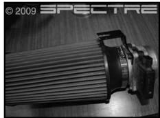
Step 12 Install the filter onto the MAFS as shown. Fully tighten the clamp.
