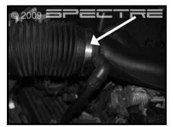
Step 3 Loosen the hose clamp connecting the stock intake tube to the throttle body.
